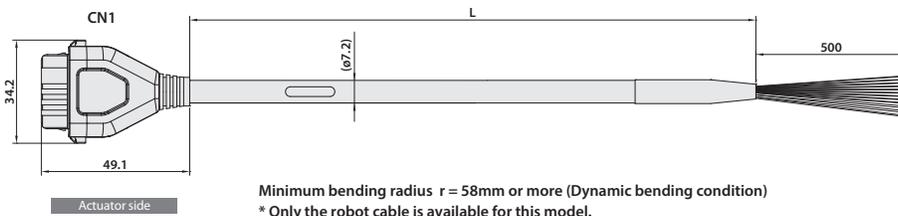
Minimum bending radius  $r = 58\text{mm}$  or more (Dynamic bending condition)
