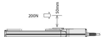
The dynamic allowable moment for EC-S7 is  $Ma = 17.7 \text{ (N}\cdot\text{m)}$ , which means it is OK since  $17.7 > 14.4$ .
