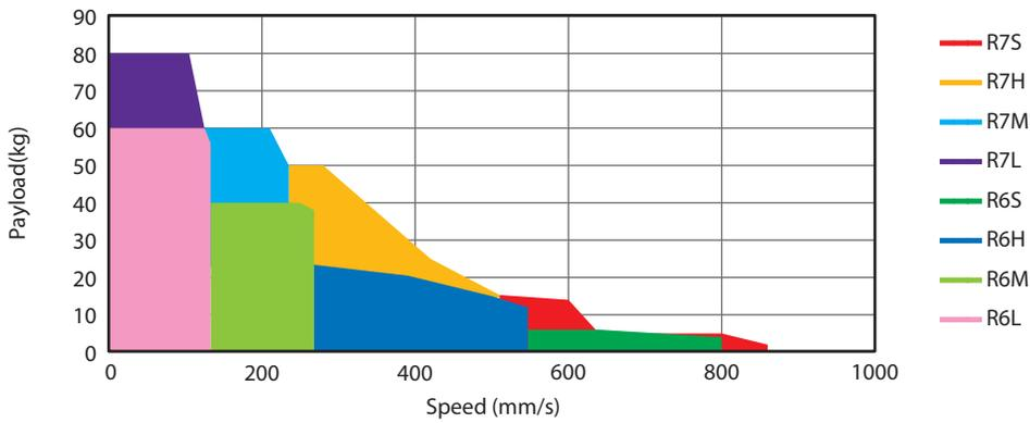
Rod Type, Vertical Mounting, Stroke: ~ 300mm
