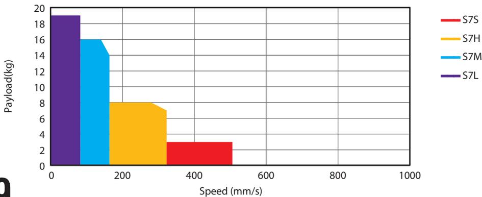
Rod Type, Horizontal Mounting, Stroke: ~ 200mm
