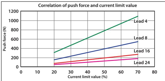
\* During push motion, the speed is fixed to 20 mm/s. If the velocity setting value (V) is less than 20 mm/s, the speed setting of V is used for the push speed but the push force will be unstable.
