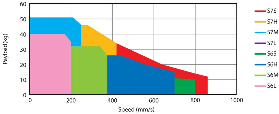
Slider Type, Horizontal Mounting, Stroke: ~ 300mm
